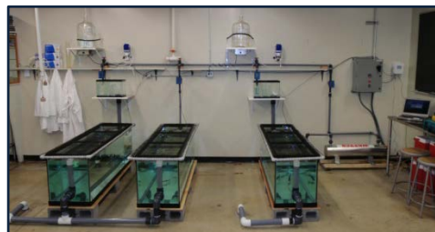
Figure 1. Flow-through freshwater herbicide exposure tanks for salmonids. Coho, Chinook and steelhead were reared in freshwater under ideal husbandry conditions before placement into flow-through tanks. Salmon were exposed to varying concentrations of endothall 0-12 ppm for 96 hours and allowed to recover before a 10-day seawater challenge assay.
